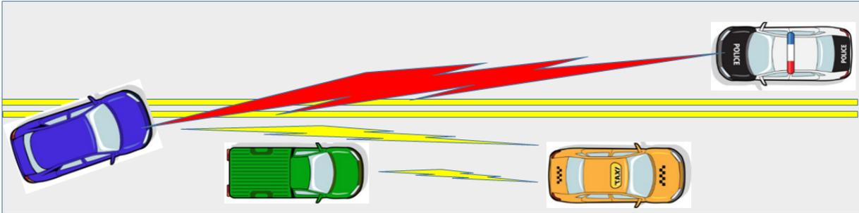
OBU from taxi transmits BSM that cab is moving slowly. OBU from blue vehicle transmits BSM that it is changing heading, potentially encroaching into pathway of police vehicle. Application Interface in police vehicle warns that blue vehicle may be encroaching into lane, while application interface in blue vehicle warns that there is an approaching vehicle (police car)
