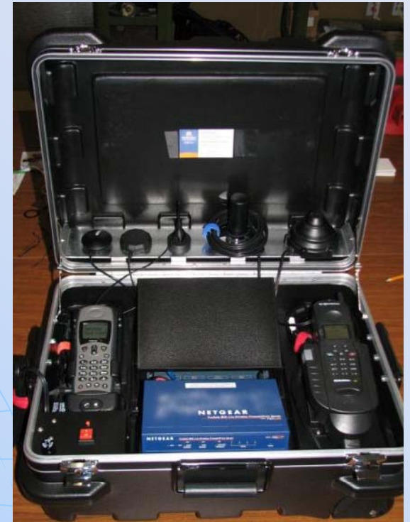
A communication box that includes GPS , Wi-Fi , Cellular and Satellite modems
